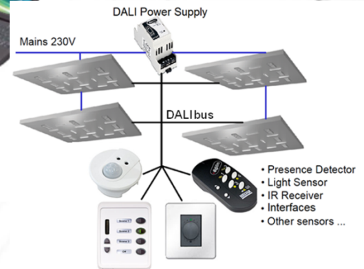
Picture 2: Standalone DALI system
